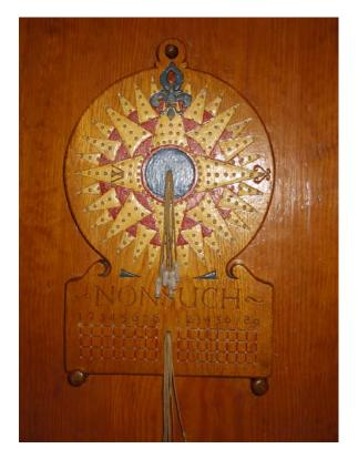
The device is called a traverse board, a memory aid, used to easily record speeds and directions sailed during a watch. Even an illiterate crew could use the traverse board.
