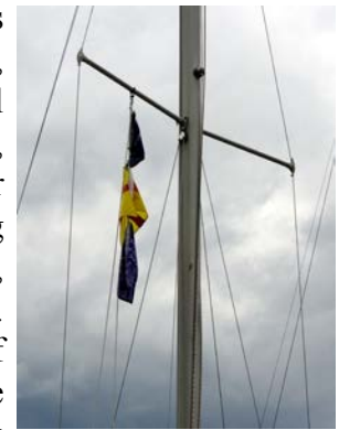
Starboard signal halyard is second in priority.
