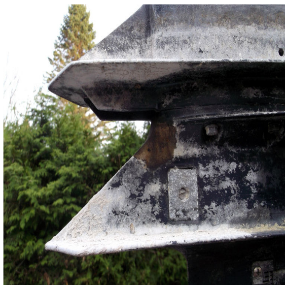
Outboards are usually equipped with a pair of anodes bolted through the lower unit, below water level.
