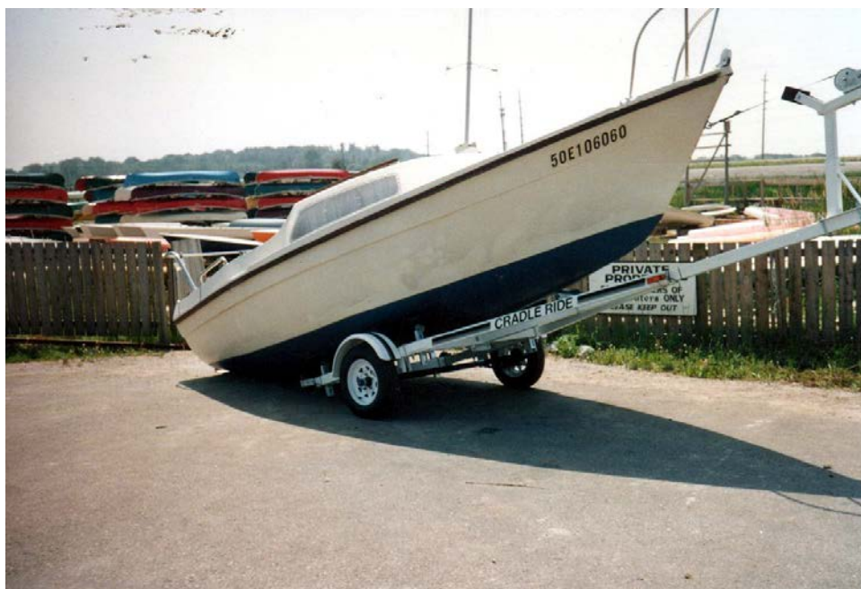
How not to load a boat! You need 8 to 10 % of the load weight on the tongue.
